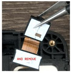
Next we will remove the rear camera. This is basically the same process. Simply unplug the camera from the board and remove. Notice in the photos that you can now see the microphones on the device as well as the light sensor. I prefer to remove these as well.
